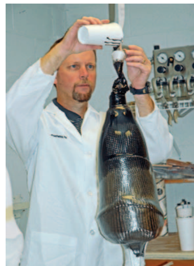
Adding catalyst-pigment mixture to activate socket lamination.
